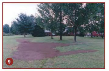
Inspect and review the absorption field area for possible drainage problems and make sure the absorption field is secure from water run-off. If necessary construct a curtain drain to divert flow away from the absorption area.
